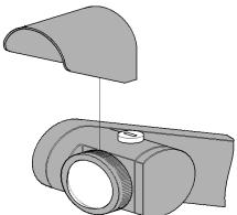
7.1.3.Adjust the arm height and oven head angle to suit by loosening the clamp screws and adjusting as required. Retighten the clamp screws after making adjustments. Always loosen the clamp screws before making adjustments.
